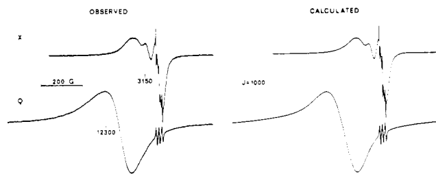
Figure 2. EPR spectra of the ortho-spin-labeled copper porphyrin V in toluene solution at room temperature. The X-band (9.11 GHz) spectrum is an 800 G scan obtained with 20 mW power and 0.63 G modulation amplitude. The Q-band (35.25 GHz) spectrum is a 1000 G scan obtained with 1.5 mW power and 2.5 G modulation amplitude. J is given in gauss. The simulated spectra include the contribution from "free" nitroxyl with a concentration 0.1% of the concentration of V.
